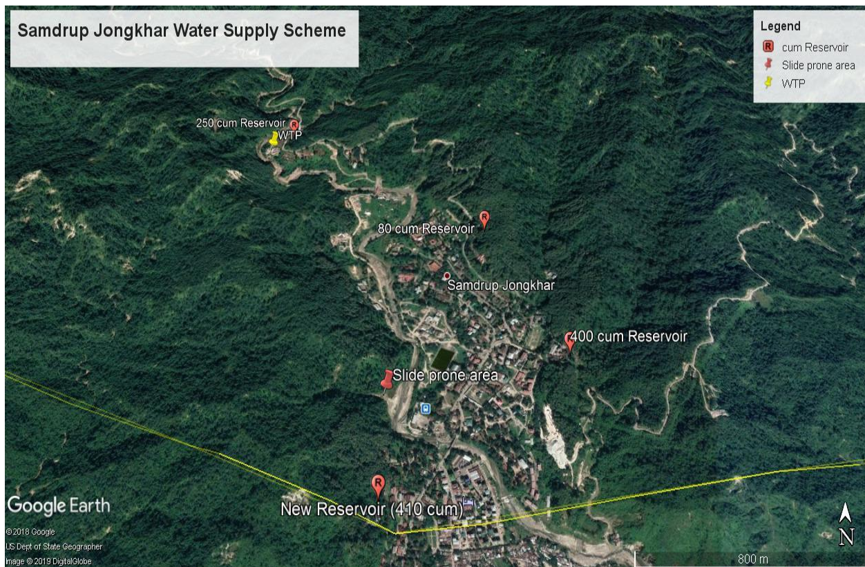
Map 8 showing locations of all Reservoirs. The new reservoir (410 cum) will be built under STUDP
